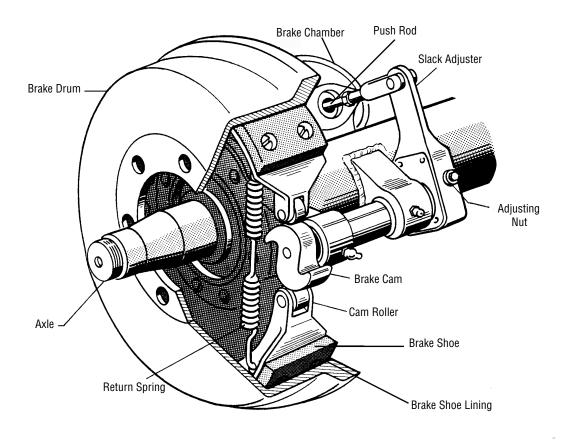
Figure 5-2 S-cam Air Brake
