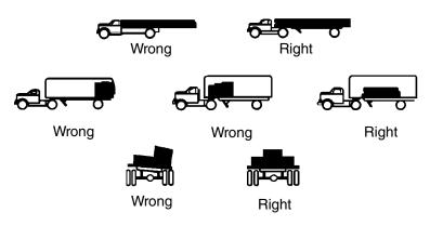
Figure 3-1 Balancing Cargo Weight
