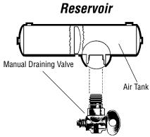
Figure 5-1 Manual Drain Valve
